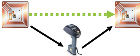
Fig. 5. Inter-Tag communication. Passive tags can communicate with each other through the reader.
