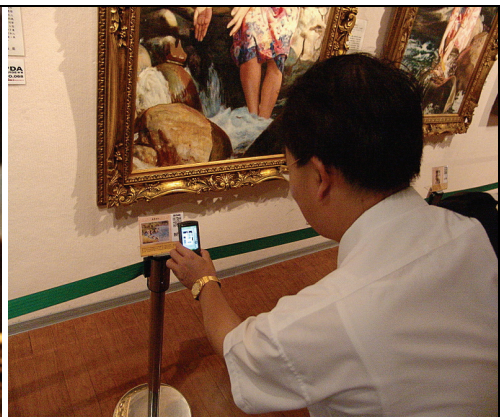
Fig. 6. The visitor moved the handheld computer close to the information plate. The RFID-reader picks up the ID of the painting.
