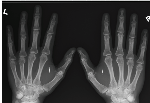
Fig. 6. An X-ray of Amal Graafstra's hand. The chip in the right hand is a Philips HITAG S 2048 and is equipped with crypto-security. Source: http://www.amal.net/rfid.html
