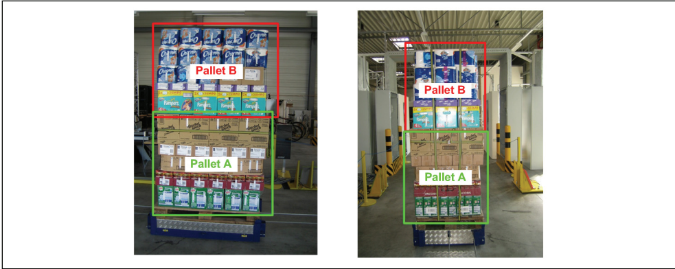
Fig. 5. Pallet with typical items often transported in a supply chain (mineral water, fish, toilet paper, toys and snacks) placed on the automated transport system
